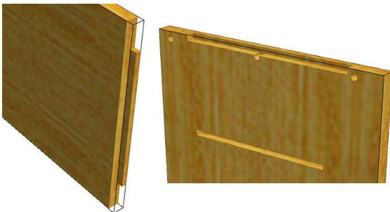
This version allows you to assemble two parts while avoiding horizontal drillings in the edges.
